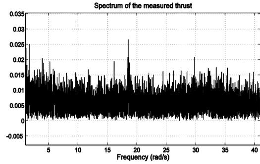
Fig. 5. Spectrum of the measured steady state thrust measurement (low frequency -less than 1rad/s- components omitted).
