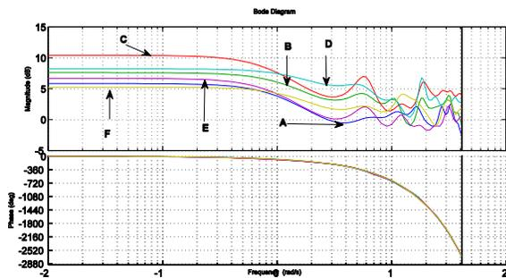
Fig. 6. Bode diagram of the identified discrete transfer functions.
