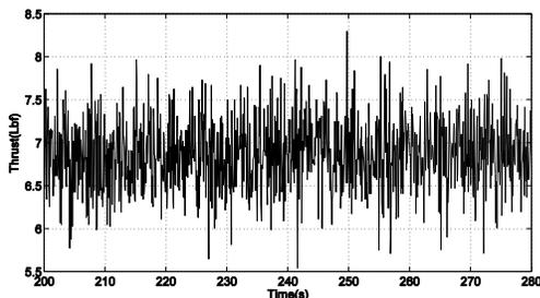
Fig. 4. Measured thrust in the constant fuel-flow experiment.
