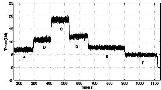
Fig. 2. Experimental thrust for the input of Fig. 1.
