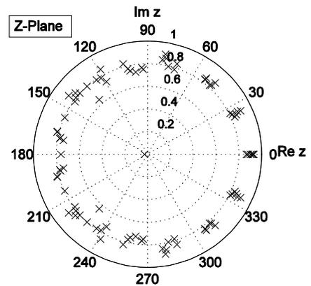
Fig. 7. Root loci of the poles of the identified discrete transfer functions
