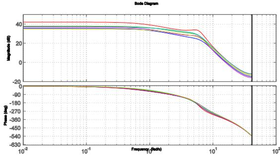
Fig. 9. Bode diagram of the reduced discrete transfer functions.
