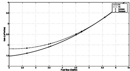
Fig. 3. Static-thrust/fuel-flow relationship.
