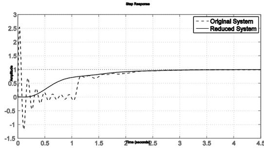
Fig. 10. Step responses of a reduced and non-reduced transfer function
